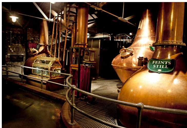
Feints Still, wash still and spirit safe (left side brass and glass box)
